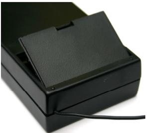
Please note we do NOT recommend the use of Zinc Carbon or standard re-chargeable batteries in the E-Stim Systems Series 1 Remote Receiver. NiMh re-chargeable batteries, with a terminal voltage of 8.4V or above may be used with a possible reduction in output power.
