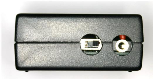
Connection to electrodes is via a single 3.5mm mono jack socket on the top of the receiver. Ensure the unit is switched off before inserting or removing the connection jacks to eliminate the possibility of either inadvertent electric shocks or short circuits occurring. Adapters are available for 2mm and 4mm connectors.
