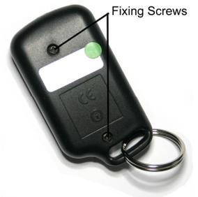
Open the case and gently remove the battery from the two clips. Insert the new battery, noting the polarity marked by a '+' on the board and the battery and close the case.
