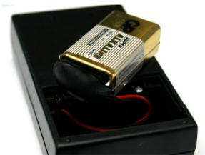
Place the battery into the unit and replace the battery compartment cover. The cover is fitted with two tabs which insert into the lower half of the case first, then the top half of the cover will then clip into position.
